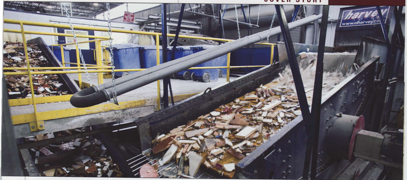
E.L. Harvey uses a water bath as part of its sorting process.
